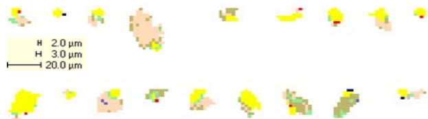
BFP-KH: Binary Cu-Sulphide and Qtz-Flds (-75/+20µm)
