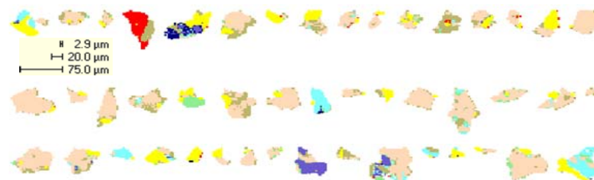
SS: Cu-Sulphide Complex (-75/+20µm)
